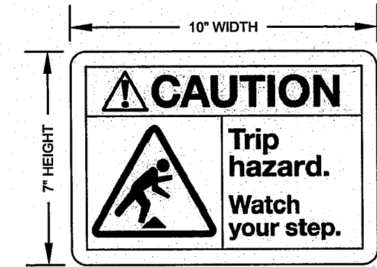
TRIP HAZARD SIGN DETAIL (IF NEEDED) SCALE: 3" = 1'-0"
