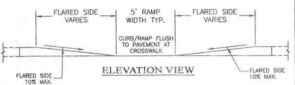
**12 DEPRESSED RAMP/DETECTABLE WARNING DETAIL**
