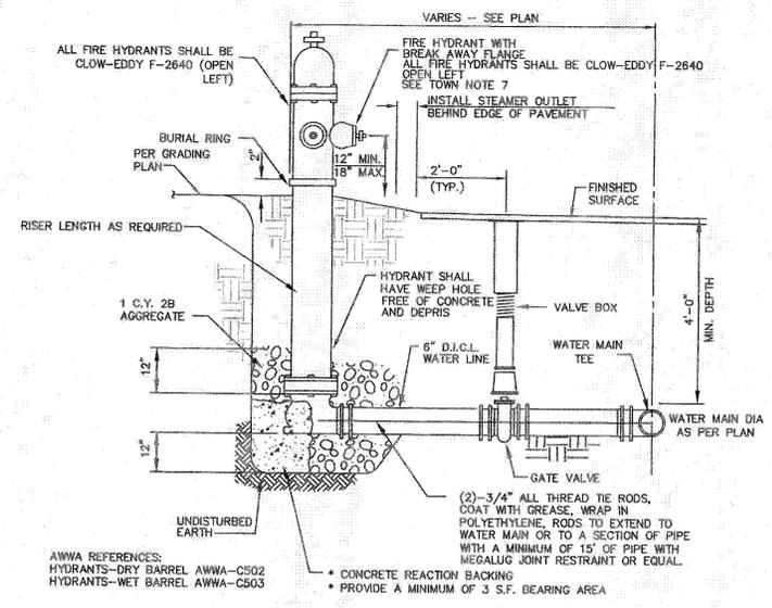
NOTE: IF HIGH GROUND WATER IS ENCOUNTERED, THE HYDRANT DRAIN HOLE SHOULD BE PLUGGED AND THE HYDRANT MARKED OR LABELED TO INDICATE THAT THE BARREL MUST BE PUMPED OUT AFTER USE TO PREVENT DAMAGE FROM FREEZING
