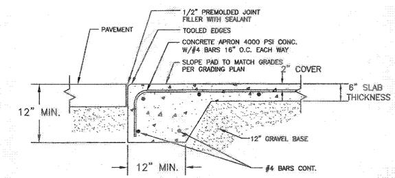
**4** DUMPSTER CONCRETE PAD DETAIL
