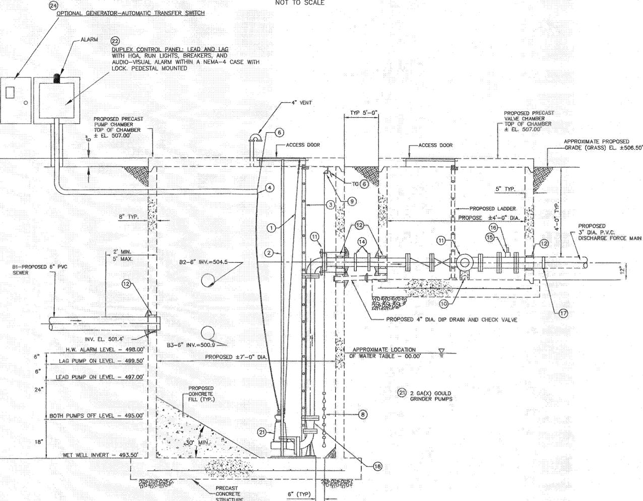
CROSS-SECTION OF PUMPING STATION AND VALVE CHAMBER
