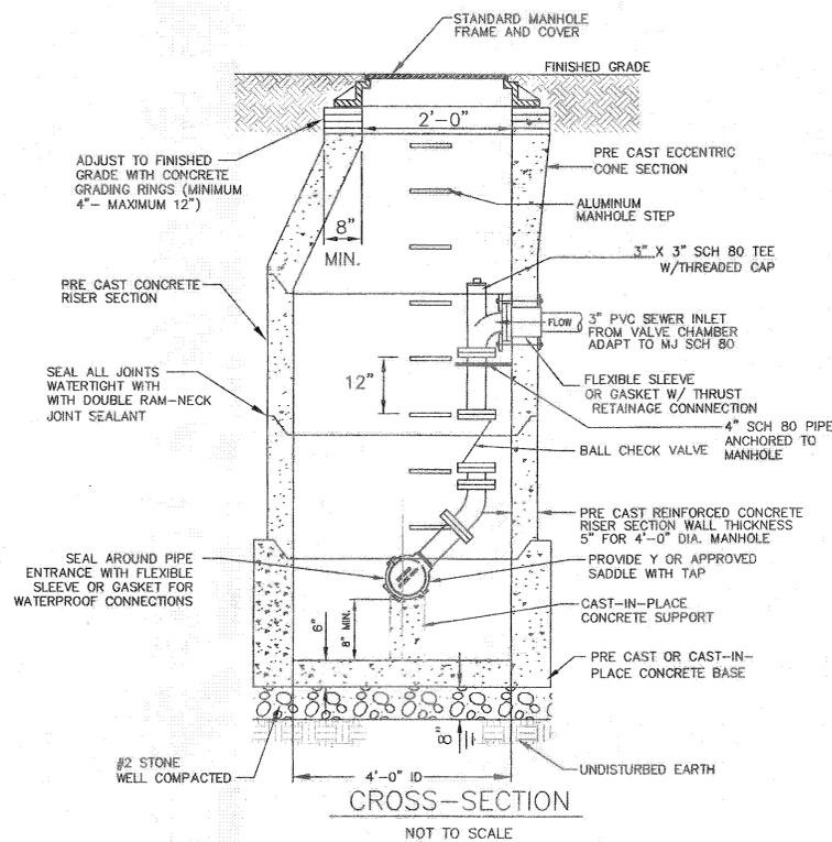
**5 SEWER MANHOLE W/ FORCE MAIN CONNECTION DETAIL**
