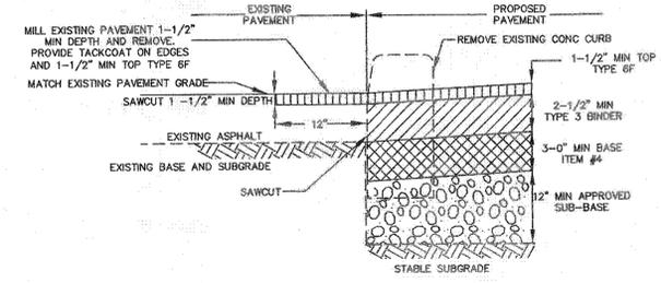
**9 TYPICAL PAVEMENT CONNECTION DETAIL**
