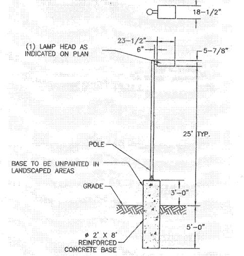
**POLE MOUNTED LIGHT DETAIL (FIXTURE A, B, AND C)**
