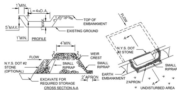
OPTION: A ONE FOOT LAYER OF N.Y.S. DOT #2 STONE MAY BE PLACED ON THE UPSTREAM SIDE OF THE RIPRAP IN PLACE OF THE EMBEDDED FILTER CLOTH.
