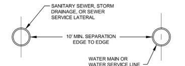
**WATER & SEWER HORIZONTAL SEPARATION**
