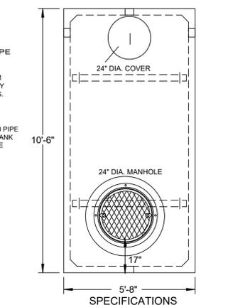
CONCRETE MIN. STRENGTH: 4,000 PSI AT 28 DAYS
