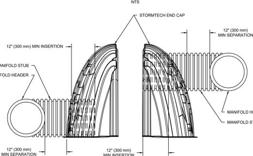
NOTE: MANIFOLD STUB MUST BE LAID HORIZONTAL FOR A PROPER FIT IN END CAP OPENING.
