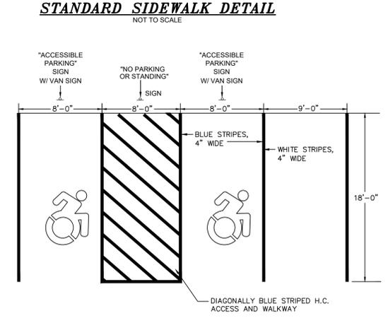
**HANDICAP AND TYPICAL PARKING SPACE STRIPING DETAIL**
