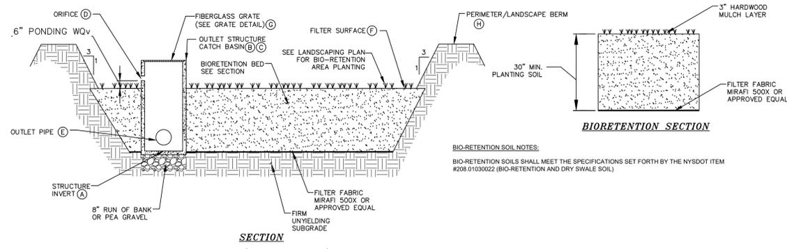
**BIO-RETENTION AREA (PR-OCS-2) DETAIL**
