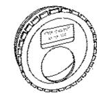
1. INSERT A SPEED LEVELER IN THE END OF ALL OUTLET. PIPES IN THE DROPBOX. 2. ROTATE UNTIL EFFLUENT ENTERS ALL OUTLETS EQUALLY.
