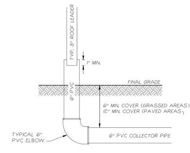
**Typical Roof Drain Detail**
