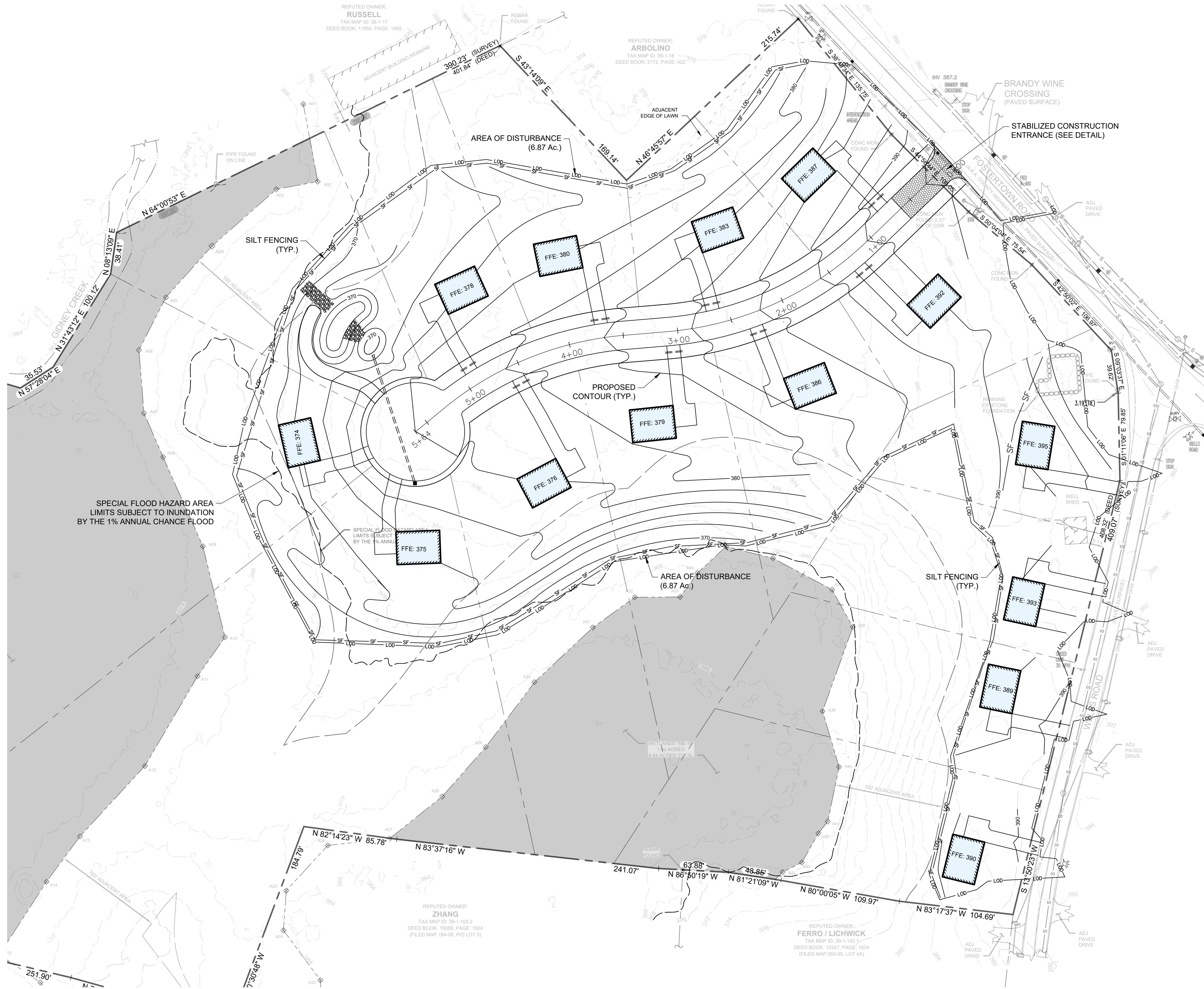
1 GRADING & EROSION CONTROL PLAN C-3 SCALE: 1"=50'
