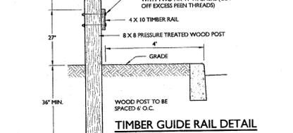
TIMBER GUIDE RAIL DETAIL N.T.S.
