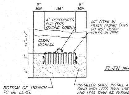
ELJEN IN-DRAIN SYSTEM CROSS SECTION
