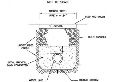
BACKFILL SHALL BE RUN-OF-BANK GRAVEL COMPACTED IN 6\"/>
